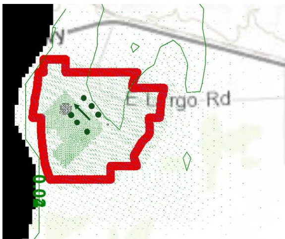
6j) Groundwater velocity contours and vectors (layer 10)
