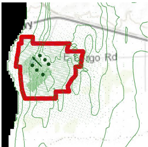
5h) Groundwater velocity contours and vectors (layer 8)
