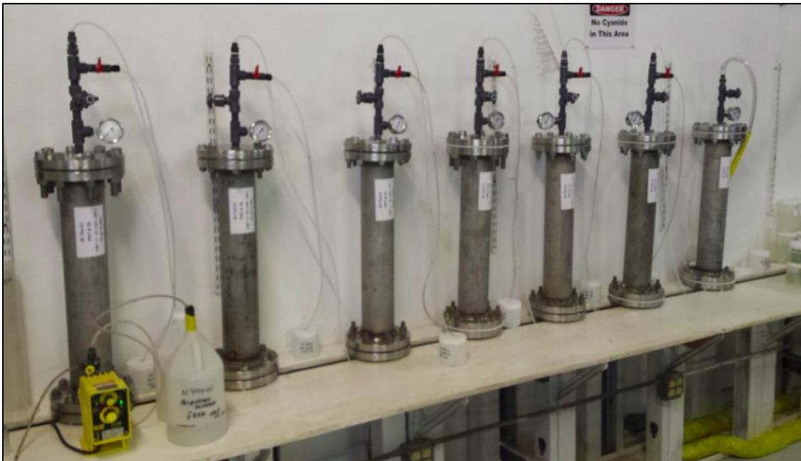
Figure 13-5: Series Leach Test Apparatus
