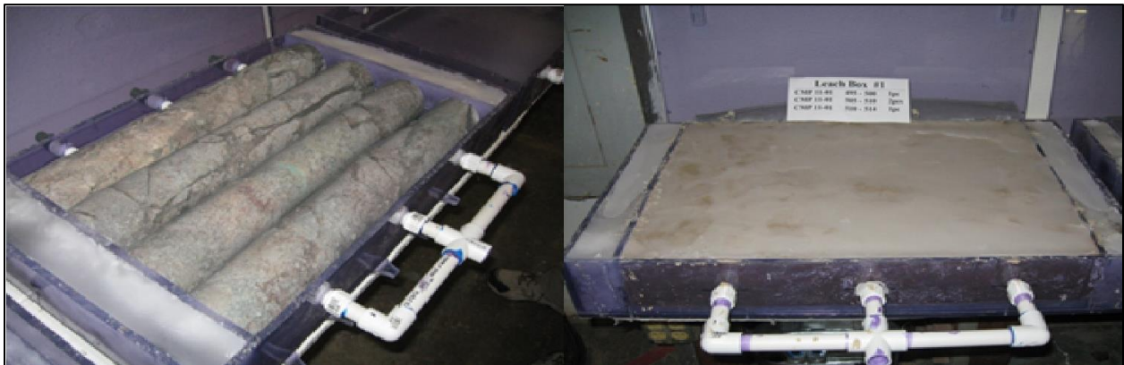
Figure 13-1: Leach Box Setup with Core Sample (Left) and Loaded with Silica Sand (Right)
